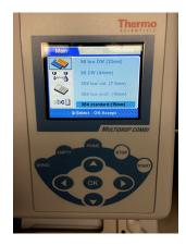
6. Next, select the volume and cassette type by highlighting the next menu option in the list (depicted with a two drops icon) and pressing the OK button. Choose the small or standard tube cassette by using the right and left arrow keys. (Unless informed otherwise, ICCB-L is providing small bore cassettes.) Set the volume using the up and down arrow keys. When finished, press the OK button.
