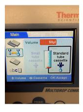
7. Choose which columns to fill by selecting the 3<sup>rd</sup> option in the list (depicted with a half full plate icon) and press OK. Choose whether to fill the entire plate or select columns. If choosing columns, use the left and right arrow keys to move and the OK button to toggle on/off. The color orange indicates the column will be filled. Move to the "Accept" button on the screen using the down arrow and press the OK button to accept these changes.
