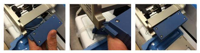
3. Next, stretch the back of the cassette (the other blue portion) under the pump, and up over the top until it is doubled over and nearly on top of the front of the cassette. The tabs should slide into the slots on the front of the Combi and keep it in place.
