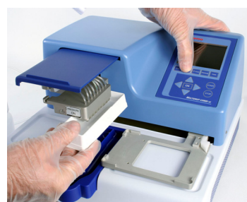
Cleaning the tubings using a reagent basin
