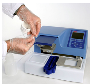
1 Removing the reagent filter
